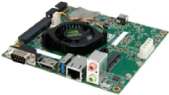
Deep Network-based computer vision on NVIDIA Jetson Tegra K1 system-on-chip wearable processing board
